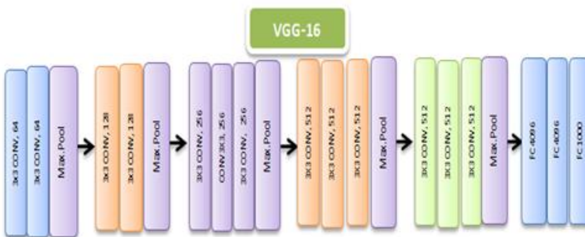
Figure 2 Architecture of VGG-16 Model
